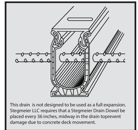
This drain is not designed to be used as a full expansion. Stegmeier LLC requires that a Stegmeier Drain Dowel be placed every 36 inches, midway in the drain to prevent damage due to concrete deck movement.
