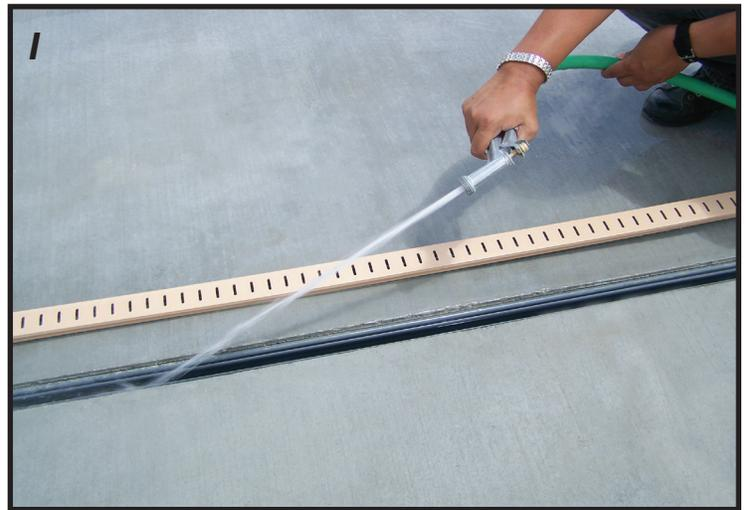
**H, I.** The top caps can be easily removed for cleaning or replacement. The top cap snaps in and out using the flex in the top cap legs. This unique attachment has no external fasteners (screws) that detract from the attractive appearance.
