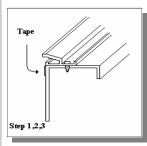
Step 1. Lay the liner track down (the bottom of the track needs to be flush with side wall). Use self-tapping screws to hold the track in place.
