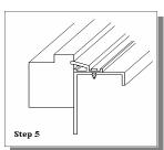
Note: On cold weather days the side of the liner should be warmed up. To do this, heat the side wall up (with a heat gun) one foot in front of the form you are about to attach.
