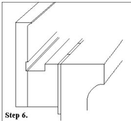
**Step 6.** Peel the paper from the face form and line the bottom of the face form up with the bottom of the extender. Press the face form to the extender.
