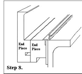
**Step 8.** End piece (the side of the pool opposite the roller). All the end pieces will be marked "END PIECE". Place the extender on (it will be upside down). Then the face form and the tile strip.
