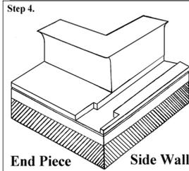
**Step 4.** Place the preformed corners in the corners opposite the roller. There is a groove cut in the corners. This groove should run parallel with the track side. Peel the brown paper on the double faced tape (one side at a time). Then line up the shelf of the corner with the tile. Press the form to the tile.
