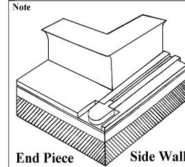
**Step 9.** Pre-drill the holes in the cover track (approximately 24 on each side of the pool). Then put a nut on the anchor, slide the anchor into the track, then put on the second nut (leave 1/8" of tread exposed after second nut). Do this for the entire track.
