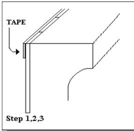
**Step 1.** Remove any burrs on top of the tile with an abrasive stone, at least 1" back from the tile. This will allow the tile strip to lay flat.
